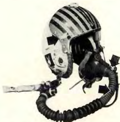
Dents on this visor cover were probably caused by the magnetic compass which broke loose. The microphone connection on the front of the mask was shattered. A hole in the O 2 hose can be seen about 4 inches from the mask. The flight surgeon stated the visor and mask protected pilot's face.
