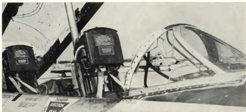
This photo shows impact point on lower right corner of right windscreen of T-33. Although considerable damage was done to the windscreen frame, the canopy was only slightly damaged.
